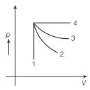
For the curve 1, volume is constant, so it is isochoric process. Between curves 3 and 2, curve 2 is steeper, so it is adiabatic and 3 is isothermal.
